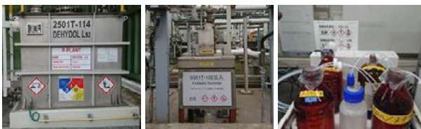
Examples of workplace GHS indication (from the left: a storage tank, raw materials intake port and analysis room)
