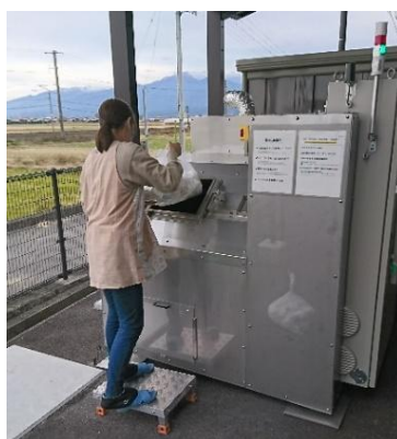
From left: the carbonization equipment developed by Kao; depositing used disposable diapers in the device; semi-carbonized material.
