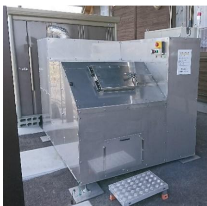
From left: the carbonization equipment developed by Kao; depositing used disposable diapers in the device; semi-carbonized material.
