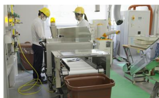
Sorting Removing packs incorporating aluminum foil
