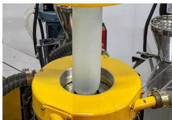
Manufacturing film Film is made in a film-forming machine. Temperature optimization controls for foreign matter, and the recycled film is ready for use.
