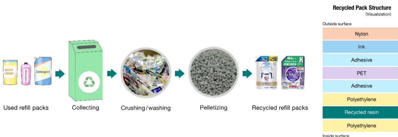
Steps to manufacturing recycled refill packs (left) and recycled pack structure (visualization, right)
