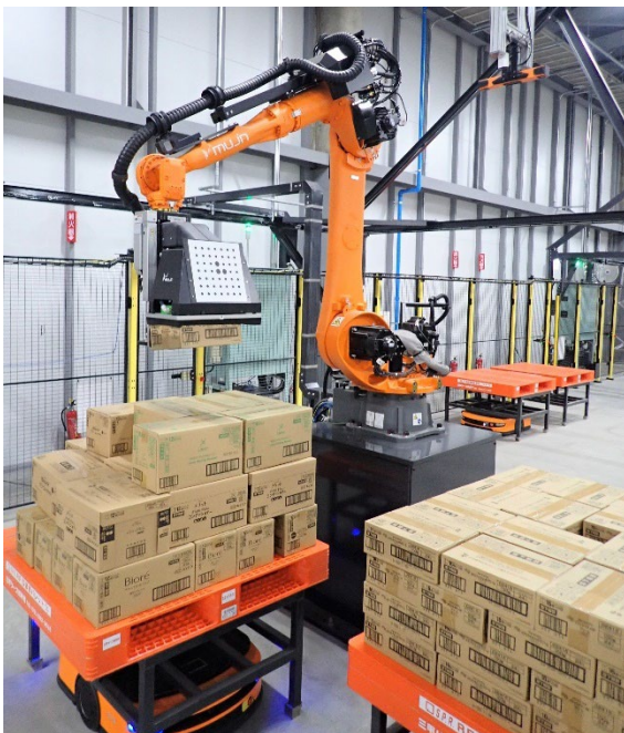
Case sorting (depalletizing/palletizing) robot
