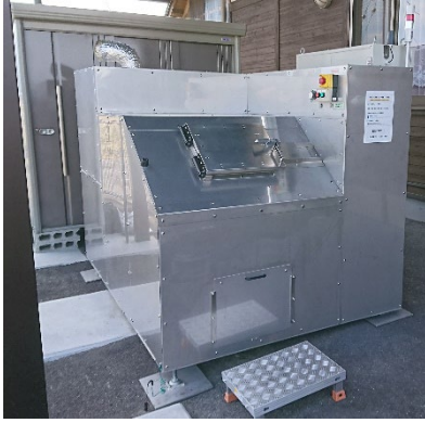
The newly developed carbonization equipment, and used disposable diapers being put into the device
