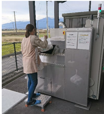
The newly developed carbonization equipment, and used disposable diapers being put into the device
