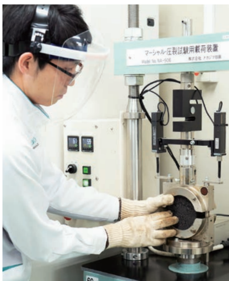
Measuring the strength of the asphalt modifier in the lab, and a paving project using the product. Adding just 1% asphalt modifier improves the durability of the asphalt pavement approximately five-fold.
