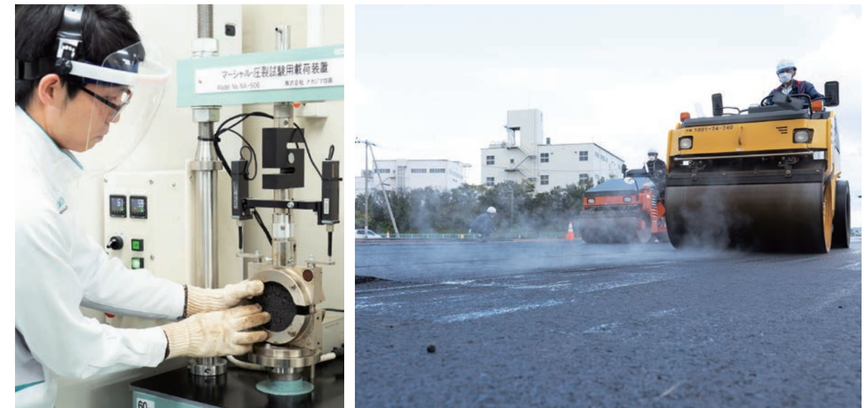
Measuring the strength of the asphalt modifier in the lab, and a paving project using the product. Adding just 1% asphalt modifier improves the durability of the asphalt pavement approximately five-fold.
