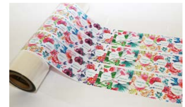
Plastic film printed using a water-based inkjet printer
